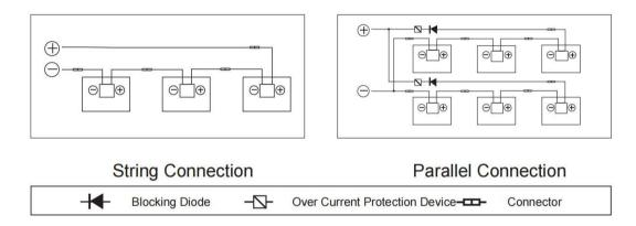
The maximum allowed quantity of modules in string connection shall be calculated according to relative regulations. The open circuit voltage value under the expected lowest temperature shall not exceed the maximum system voltage value allowed by modules and other values required by Dc electric parts. (HORAY modules maximum system voltage is DC1000V/ DC 1500V, actually system voltage is designed based on the selected module and inverter model.)
