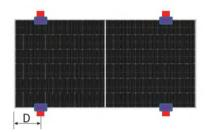
Clamps mounting (Mounting rails cross the long frame)
