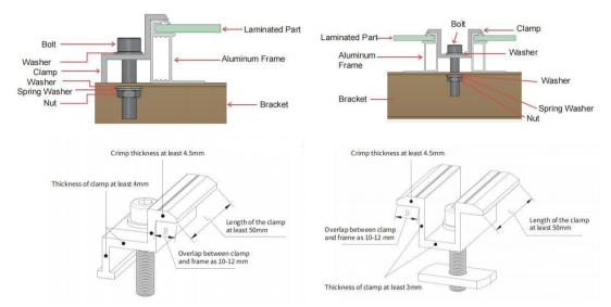
Under no circumstances should the clamp touch the glass or deform the frame. the interface of the clamp to the front of the frame must be smooth and flat to prevent frame or other components from being damaged.
