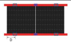
Clamps mounting (Mounting rails parallel the long frame)
